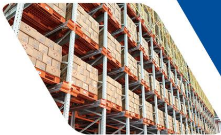
货架系统 Racking system
